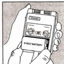
4. Insert the battery according to the diagram inside the battery compartment, making sure that the terminals are properly aligned. Make sure the lift-out tape is beneath the battery for easy removal next time.
