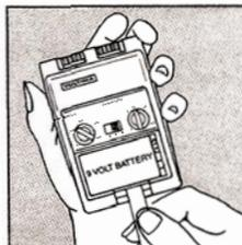
3. Remove the old battery by lifting up on the end of the lift-out tape, which should be beneath the battery.
